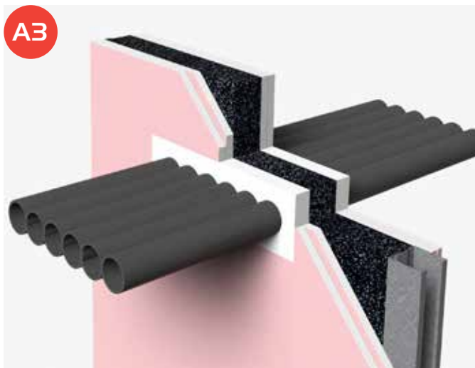
FZ100 Fire Safe Zone and row of combustable pipes
