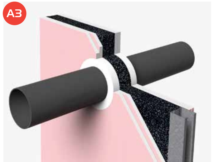
FZ100 Fire Safe Zone and combustible pipe
