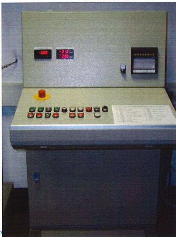
Figure 3a: Test bench control (pressure control)
