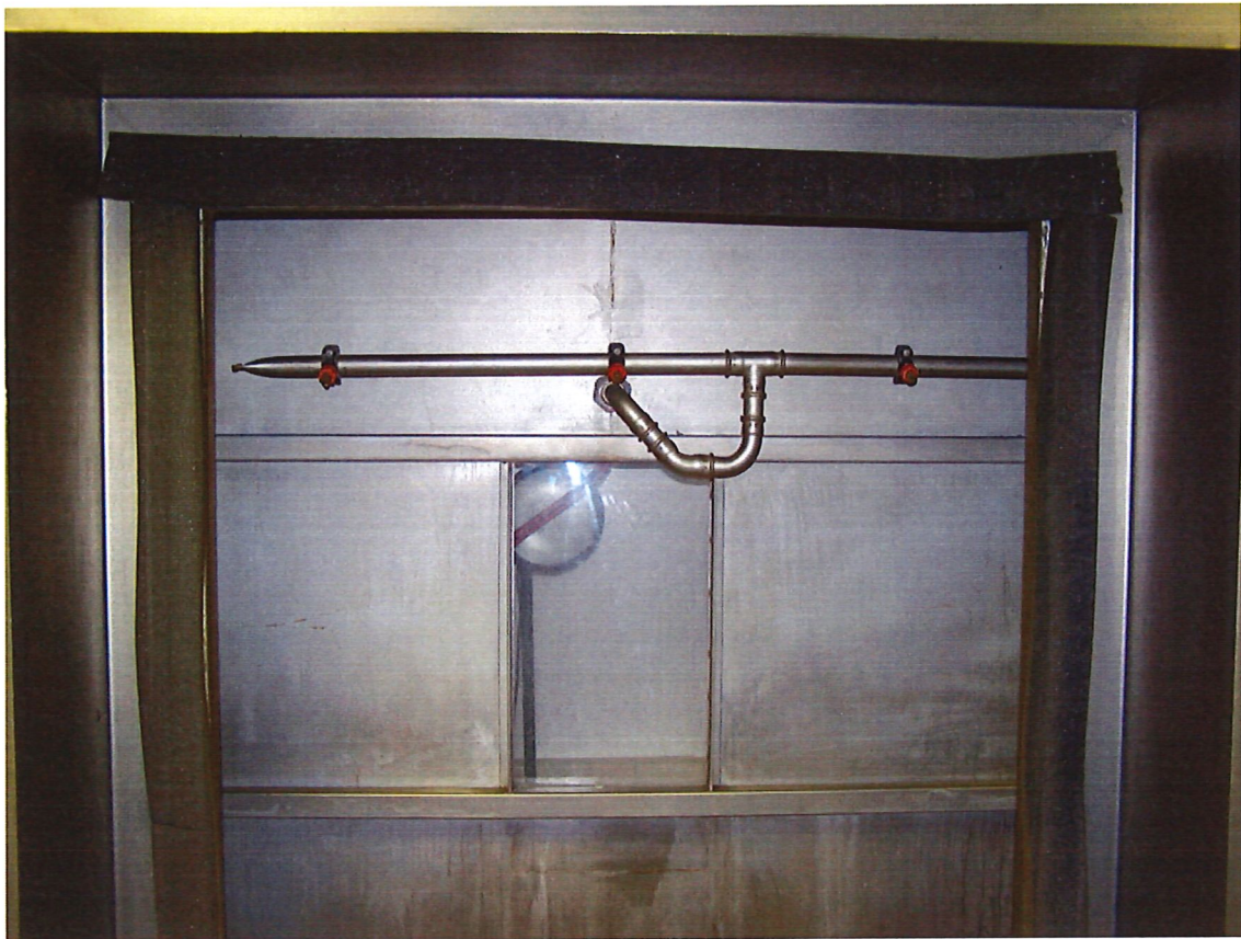
Figure 2: Open test bench with arrangement of the three water spray nozzles
